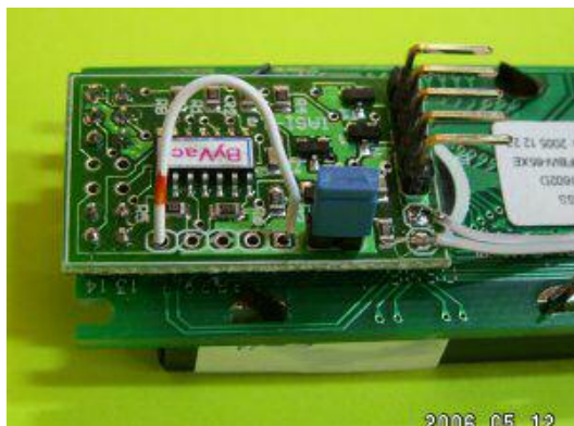
Figure 5 Shorting link as on a BV4103
