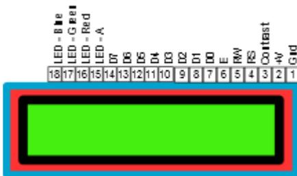
The RGB Back light type display has 18 pins to accommodate the two extra back lights.
