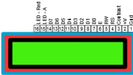
The standard LCD display has 16 pins as shown above. The 'red' output is used to vary the brightness of the back light.
