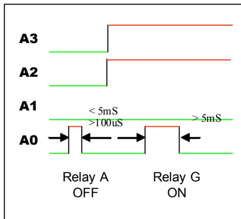
The timing for the clock pulse is very flexible in that any length of clock less than 5mS will turn the relay off and any longer then 5mS (even 1 or 2 seconds) will turn the relay on.
