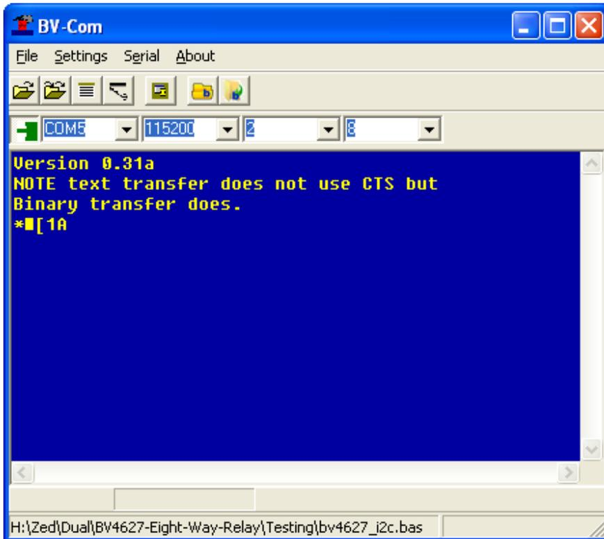
As the escape is a none printable character it looks like a square on BV-COMM. It is a good idea to get used to the commands using BV-COMM before programming.
