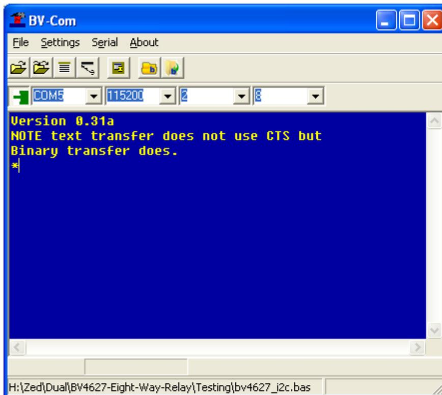
The '\*' is the response from the device to indicate that it is ready to accept commands.
