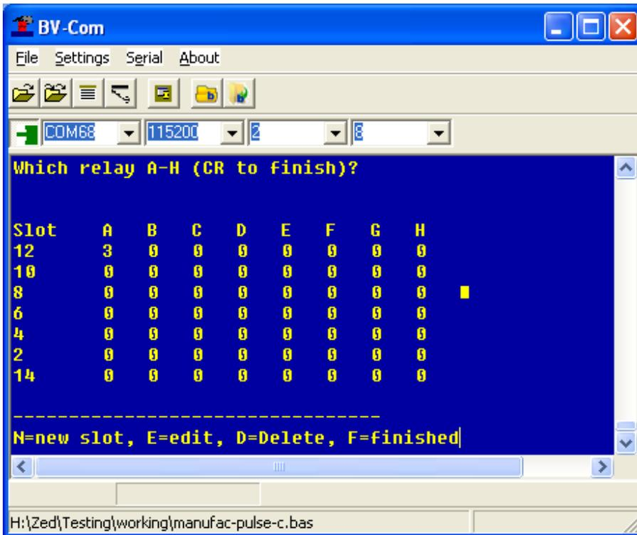
See how relay A has now been set to 3. All of the other functions can be set up in this way
