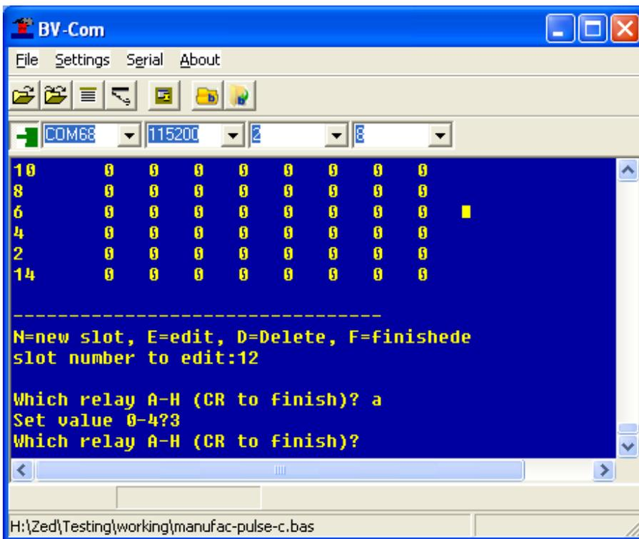
The Edit function will ask which slot, this should be the slot number, in this case 12. when this has been entered you are asked for a relay, enter 'a' through 'h' to select the relay of interest and then put in a number form 0 to 4. The number 3 will have the effect of toggling this relay. As we want this button only to control one relay press CR and you will be taken back to the map menu:
