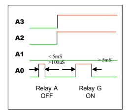
The timing for the clock pulse is very flexible in that any length of clock less than 5mS will turn the relay off and any longer then 5mS (even 1 or 2 seconds) will turn the relay on.
