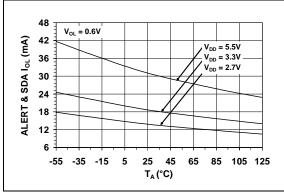
**FIGURE 2-7:** ALERT and SDA I<sub>OL</sub> vs. Ambient Temperature.
