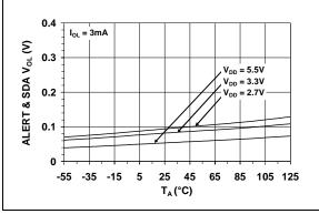
**FIGURE 2-8:** ALERT and SDA Output V<sub>OL</sub> vs. Ambient Temperature.
