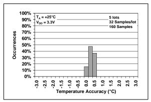
**FIGURE 2-4:** Temperature Accuracy Histogram,  $T_A = +25^{\circ}$ C.
