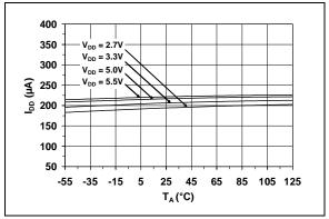
FIGURE 2-5: Supply Current vs. Ambient Temperature.
