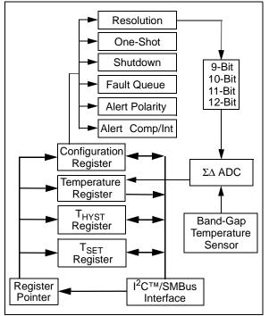
FIGURE 4-1: Functional Block Diagram.
