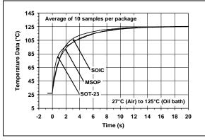
FIGURE 2-9: MCP980X Thermal Response vs Time.
