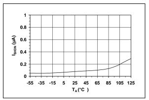
FIGURE 2-6: Shutdown Current vs. Ambient Temperature.
