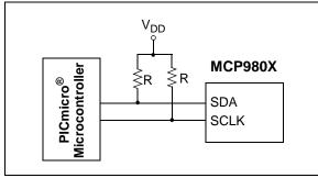
FIGURE 6-1: Pull-up Resistors On Serial Interface.
