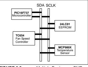
FIGURE 6-2: Multiple Devices on SMBus.
