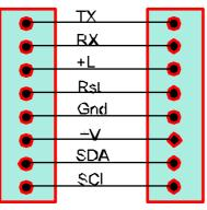
The +L pin goes to pin 20 of the IC and is therefore the main supply. The +V pin does not go to any part of the IC.
