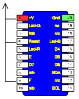
For correct operation Pins 4 and 9 must be tied to +V.
