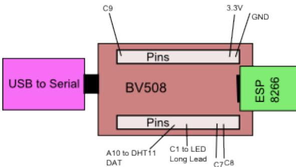
The block diagram shows the location of the pins. To maximise the room of the breadboard. The BV509 has the pins soldered upwards and connections are made with M-F connectors.
