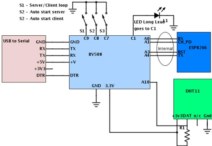
This is the circuit diagram. The three switches are not really switches but juts wire links to the breadboard. Note also that the ESP8266 is part of the BV508 and so does not need wiring.
