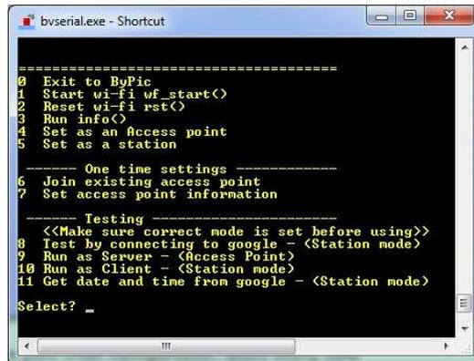
This is the main menu when S1 to S3 (jumpers) are open (not connected to ground). From here the Wi-Fi module can be manipulated.
