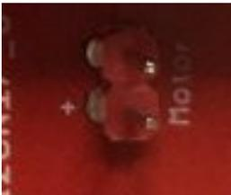
GND Motor ground pin
