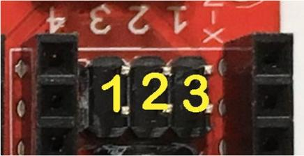
There are three jumpers per motor designated as above, this controls the step rate for each motor
